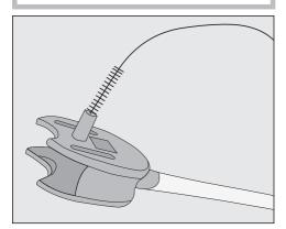
Use the brush to clean the rinse valve body under running water to remove any milk residues.
