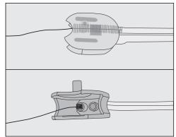
Clean also the hose connections in the rinse valve body. To do this, insert the cleaning brush into both openings and move the brush back and forth.
