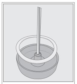
If necessary, you can remove the connecting piece and sealing ring from the milk flask lid. Once you have removed the stainless steel tube, the connecting piece is easy to push out from the inside of the lid. Clean the individual components in a dishwasher.
