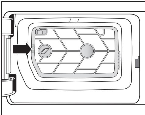
③ Press the frame of the filter insert in at the positions marked PUSH until it audibly engages.
