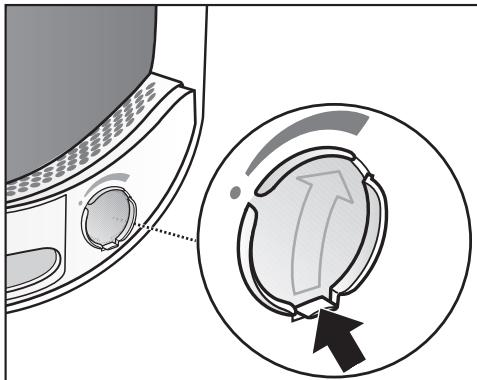
If you are not using a fragrance flacon: push the tab down completely (see arrow) so that the socket is closed. Otherwise, fluff will accumulate here.
