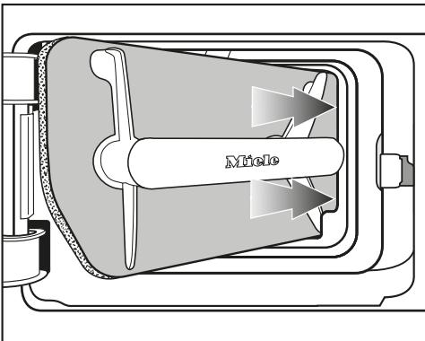
① Use the handle to slide the fluff filter on the right at an angle behind the edge.
