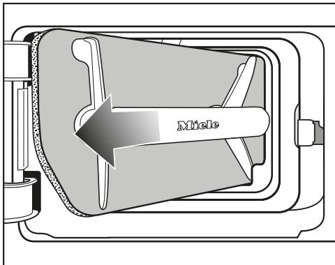
② Pull the plinth filter out at an angle.
