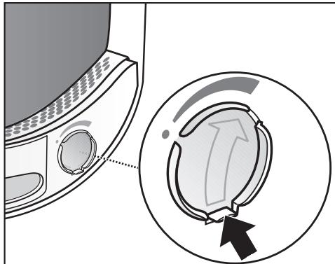
■ Open the cover using the tab until the tab is right at the top.
