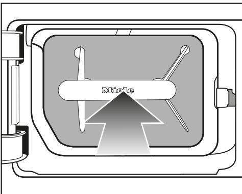
② Then press on the handle until the fluff filter is secured in position.
