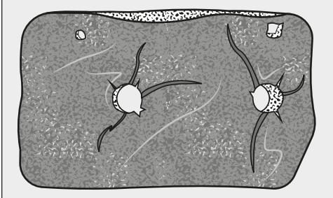
Fluff will blow into the heat exchanger through cracks and tears and will cause obstruction.
