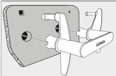
■ Pull the handle out of the plinth filter.
