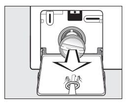
■ Remove the drain filter completely.
