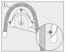
Attach the elbow ② to the drain hose ①.
