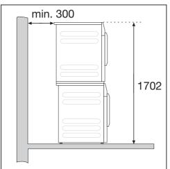
This washing machine can be installed with a Miele tumble dryer on top of it. This requires a Miele washer-dryer stacking kit which can be purchased separately.
