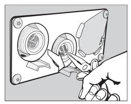
■ Withdraw the filter at the bar with pointed pliers and rinse it clean under running water. Reassemble the filter and seal in the reverse order and reconnect the hose.
