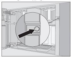
There is a red silicone plug inside the screw hole which secures the appliance door during transport to prevent transport damage.
