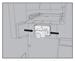
Press the catches on the left and right-hand sides of the milk valve holder and pull the holder forward to remove it.
