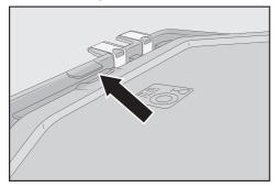
Attach the drip tray lid as follows: slide the lid under the lug next to the contacts and apply pressure to the lid until the catches at the sides audibly click into place.
