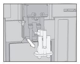
Grip the dispensing unit by the sides and pull it down to remove it.
