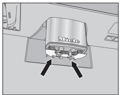
Press the two catches together (see arrows). The cup rim sensor is released.
