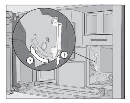
■ Press the button under the handle of the brew unit ① and, while doing so, turn the handle forward ②.
