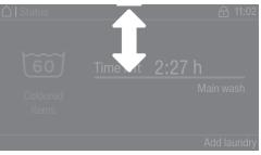
If an orange bar appears at the top of the screen in the middle of the display, you can open the pull-down menu. Touch the bar and drag down with your finger.
