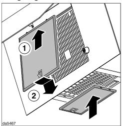
■ Insert the grease filters.
