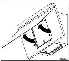
■ Pull the deflector plate out of the holder at the bottom and swing it upwards.
