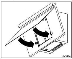
■ Swing the deflector plate downwards. It is held in place by magnets.
