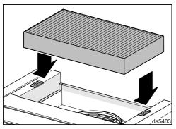
■ Fit the charcoal filter into the holder in the top of the cooker hood.
