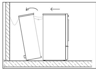
Now carefully tilt the heat-pump forwards again so that the clamping lug hooks in behind the bevelled edge on the tumble dryer.
