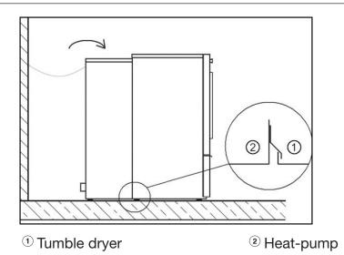
The clamping lug connects the heat-pump to the tumble dryer. Once this step is complete, the tumble dryer should no longer be able to move away.
