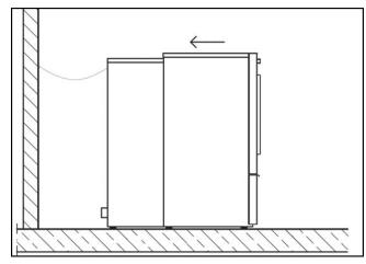
Tilt the heat-pump backwards slightly and move the tumble dryer towards the heat-pump until the lower clamping lug on the heatpump is above the lower bevelled edge on the tumble dryer.
