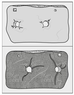
Lint will blow into the heat exchanger through cracks and tears and will cause obstruction.
