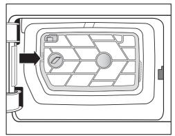
Press the frame of the filter insert in at the positions marked PUSH until it audibly engages.
