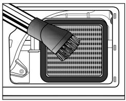
Carefully vacuum up any visible lint or soiling. Use a dusting brush or the narrow crevice nozzle.
