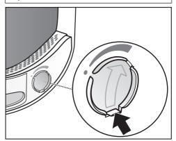
Push the tab down completely (see arrow) so that the socket is closed. Otherwise, lint will accumulate here.
