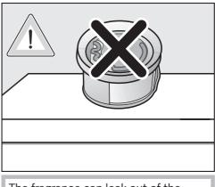
The fragrance can leak out of the capsule. Do not lay the fragrance capsule down.
