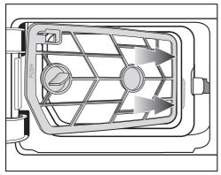
Use the handle on the right to slide the filter insert <u>at an angle</u> behind the edge.
