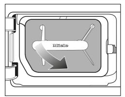
Use the handle to pull out the lint filter <u>at an angle</u> forwards and to the right.
