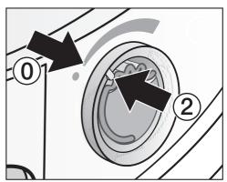
■ Turn the outer ring counterclockwise until marker ② is in position ③.
