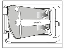
Use the handle on the right to slide the lint filter <u>at an angle</u> behind the edge.
