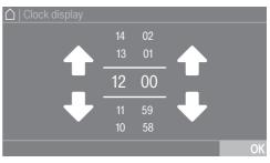
Enter the numbers by swiping upwards or downwards. Place your finger on the number that you want to change and move your finger in the direction you want. Use the OK sensor control to accept the set numerical value.
