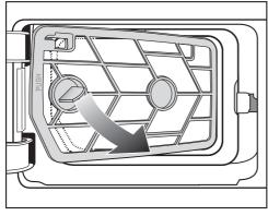
Use the handle to pull out the filter insert <u>at an angle</u> forwards and to the right.
