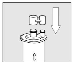
**Tip:** You can seal the descaling cartridge with the cap that can be found on the cartridge. This cap can be easily detached by snapping it off.
