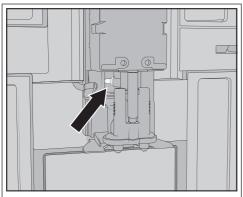
Do **not** remove the milk pipework connecting piece.
