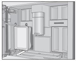
Remove the maintenance container on the left-hand side.
