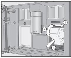
■ Pull the brew unit to the side ① first and then pull out to the front ②. Tilt the brew unit forward ③. If you cannot remove the brew unit or can only do so with difficulty, the brew unit drive is not in the correct position.
