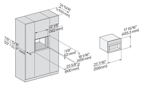
Combination with other Miele built-in appliances is possible. If the coffee machine is to be built in above another appliance, there must be a full-width, closed shelf between them. If the appliance is to be combined with a Gourmet warming drawer/ built-in vacuum drawer, no shelf is required in between.
