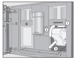
Pull the brew unit to the side ① first and then pull out to the front ③. Tilt the brew unit forward ②.
