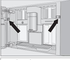
2 TX20 (25 mm) screws are supplied with the appliance.
