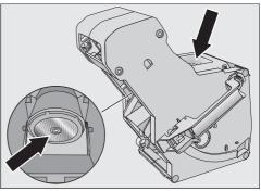
Wipe any remaining coffee off the two filters. One filter is located in the funnel and the other to the left of the funnel.
