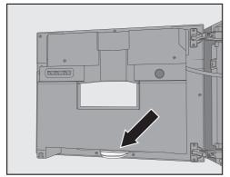
The drip tray is located at the bottom on the inside of the appliance door. Clean the drip tray regularly.
