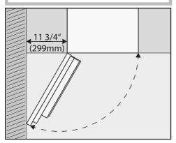
**Tip:** If a gap of at least 11 <sup>3</sup>/<sub>4</sub>" (299 mm) is maintained between the wall and the coffee machine, you will be able to open the appliance door wider, making the machine easier to use. For instance, it will be easier to remove the left-hand bean container.
