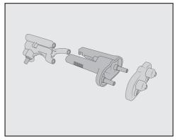
Take the dispensing unit apart, separating it into 3 components: the Y-piece, the spouts, and the holder.
