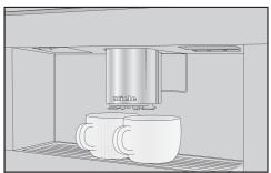
Place a cup under each of the dispensing spouts in the central spout.  Tap the sensor control immediately before or after you start making a drink.
