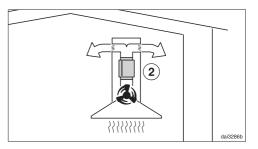
In recirculation mode, the silencer needs to be positioned between the exhaust socket and the directional unit ②. Check that there is sufficient space.
