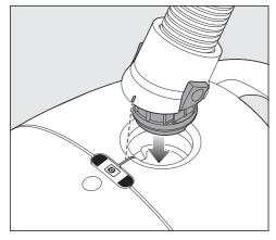
Insert the hose connector into the suction opening on the vacuum cleaner until it clicks into position. To do this, line up the guides on the two pieces.
