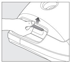
Press the release button in the recessed grip for the dust compartment lid and raise the lid as far as it will go.
