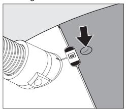
■ Press the release button on the accessories compartment lid.
