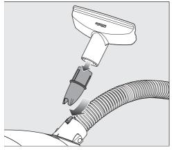
Attach the accessories holder to the hose connecter socket on the vacuum cleaner if necessary. Make sure it clicks into position.
