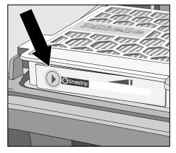
■ If you are using exhaust filter **c**, **d** or **e**, you must activate the timestrip<sup>®</sup> filter change indicator.
