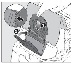
■ Insert the new vacuum cleaner bag into the raised vacuum cleaner bag holder as far as it will go. Leave the vacuum cleaner bag folded up when you take it out of the packet.
