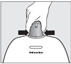
Press the release buttons at the side of the hose connector, and lift the hose from the suction opening.
