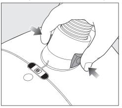
Press the release buttons at the side of the hose connector and pull the hose out of the suction opening.
