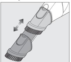
Press the release button on the dusting brush and push the brush out until it clearly engages in position. When you have finished dusting press the release button and push the dusting brush back into its original position until it clicks into place.
