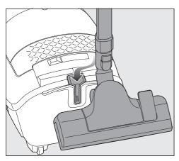
Slot the floorhead into the park system on the vacuum cleaner.
