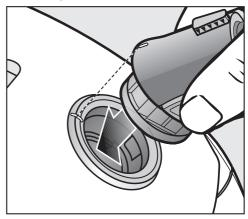
Insert the hose connector into the suction opening on the vacuum cleaner until it clicks into position. To do this, line up the guides on the two pieces.
