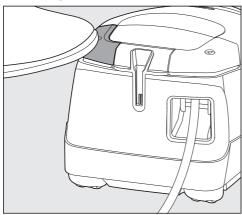
■ Press the On/Off foot switch ①.
