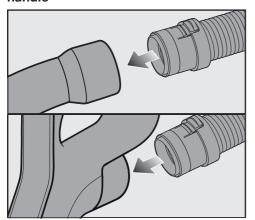
■ Fit the suction hose connector into the handle until it clicks into position.
