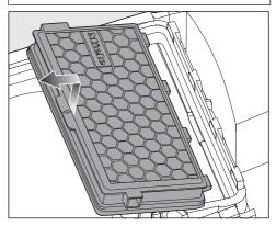
■ Lift the exhaust filter and remove it.
