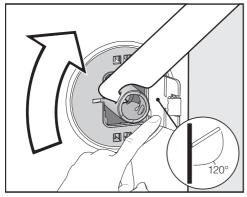
Push the cover out and turn the lefthand transit bar 90° using the open spanner supplied.
