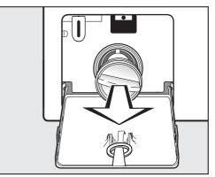
Remove the drain filter completely.
