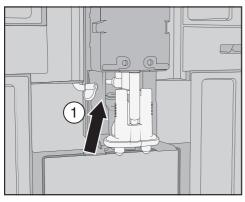
Release the milk pipework from the dispensing unit: to do this, pull the lug 1 to the left.
