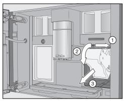
Pull the brew unit to the side ① first and then pull out to the front ③. Tilt the brew unit forwards ②.
