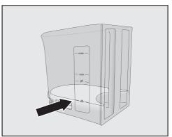
Fill the water container to the ////\marker with lukewarm water and stir the solution.
