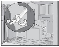
Press the button under the handle of the brew unit ① and, whilst doing so, turn the handle to the rear ②.
