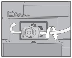
**Useful tip:** If necessary, turn the milk pipework on the right connecting piece towards the back.
