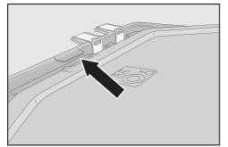
Refit the lid of the drip tray: push the lid in under the lip next to the contacts and press down on the lid until the latches click into place.
