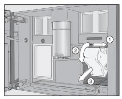
Pull the brew unit to the side ① first and then pull out to the front ②. Tilt the brew unit forwards ③.
