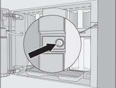
There is a red silicone plug inside the screw hole which secures the appliance door during transport to prevent transport damage.
