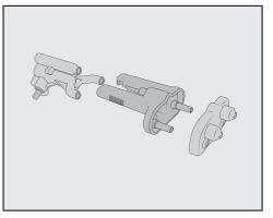
Dismantle the dispensing unit into three pieces: disconnect the Yshaped piece, the dispensing spouts and the holder from one another.
