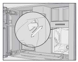
Push the slide control one setting to the front (for finer grinding) or to the back (for coarser grinding).
