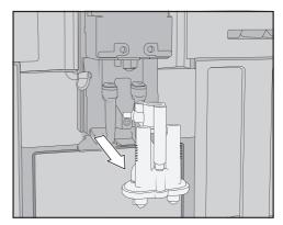
Hold the dispensing unit on either side and pull down to remove it.
