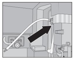
Connect the angular moulded hose to the longer milk pipework. Start by fitting the moulded hose to the top of the central spout. The black connecting piece should point towards the rear.
