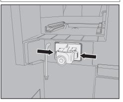
Press the catches on the left and right of the milk valve holder and pull the holder forwards to remove it.
