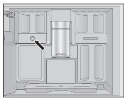
The milk valve is located under the bean container on the left-hand side.
