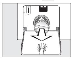
■ Remove the drain filter completely.
