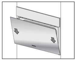
Hold the door securely on both sides and carefully install it back into the hinge retainers.
