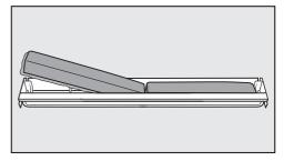
Remove both charcoal filters and place the new filters with the surrounding edge pointing downwards in the holder.
