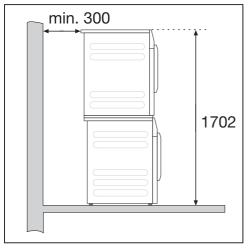
The washing machine can be installed as a washer-dryer stack together with a Miele tumble dryer. This requires a Miele washer-dryer stacking kit which can be purchased separately. ⚠️ Installing the washer-dryer stack on a Miele plinth is not permitted.
