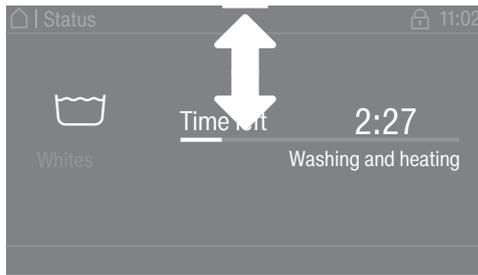
If an orange bar appears at the top of the screen in the middle of the display, you can open the pull-down menu. Touch the bar and drag it down with your finger on the display.
