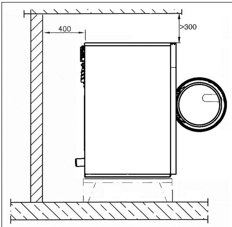
Minimum safety distance to the wall approx. 400 mm to allow for maintenance.
