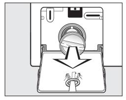
■ Remove the drain filter completely.
