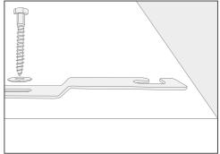
■ Install the holding bracket with the hexagon screws and the washers.
