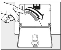
Push the emergency drain lever downwards and hold until no more water runs out.
