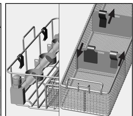
For each colour, attach one tag to the ring holders or the load item carriers and one tag to the small parts basket compartments.
