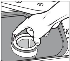
■ To unscrew the micro-fine filter, turn twice counterclockwise.
