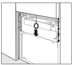
Remove the service panel and pull the ring of the emergency door release down.
