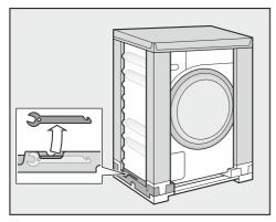
■ Take out the open-end spanner for removing the transit bars from the bottom left of the transport packaging.
