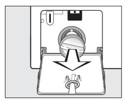
■ Remove the drain filter completely.
