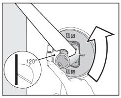
■ Push the flap outwards and turn the transit bar 90° using the enclosed spanner.
