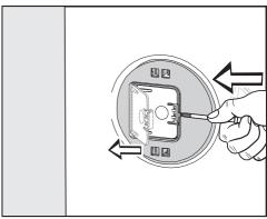
Push against the catch with a pointed object, e.g. a narrow screwdriver.
