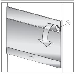
Insert the opener ① included with the appliance about 3 cm into the gap between the door and the control panel on the right-hand side and then pull the door open.
