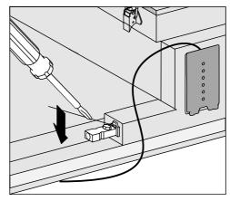
■ Loosen the lug and pull the plug out.
