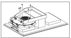
■ Undo the 5 screws on the fan.
