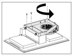
■ Slide the frame outwards towards the current extraction direction and tilt up to remove one side. Then slide in the opposite direction to remove the entire frame and fan. Then turn both 180°.
