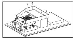
■ Undo the 4 screws on the frame.
