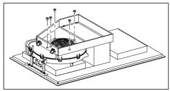
■ Undo the 5 screws on the fan.
