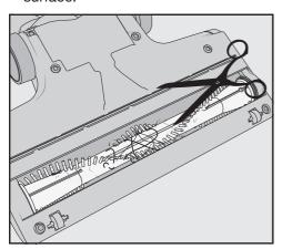
Cut any threads or hairs that have wound themselves around the roller brush with a pair of scissors. To guide the scissors, move along the guide track on the roller brush. Then run the vacuum cleaner to vacuum up the cut threads and hairs.
