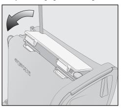
Refit the cover and lock the cable compartment.
