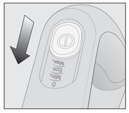
■ Press the On/Off switch on the Comfort handle (1).
