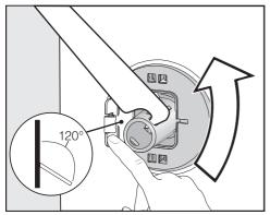
Push the cover out and turn the lefthand transit bar 90° using the spanner supplied.
