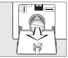
■ Remove the drain filter completely.
