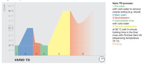
Miele recommends the use of fully demineralised water in the final rinse in order to protect the load and the washer-disinfector against stains and deposits and to protect anodised aluminium.
