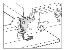
Release the locking clamps on the hinges by pushing them down. Turn them as far as they will go in an angled position.
