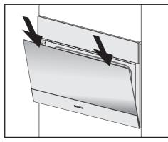
Using two hands placed on the upper edge of the door, push the door downward briefly.
