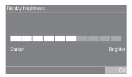
■ Touch the segment bar for the required level of brightness.
