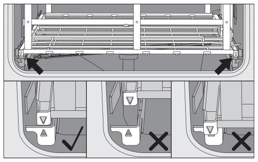
The markings on the load carrier  $\mathbf{\nabla}$  and in the wash chamber  $\mathbf{\Delta}$  must line up correctly.
