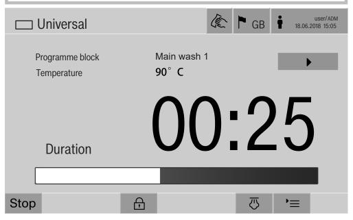
After the reprocessing programme has started, an additional **b** button is displayed next to the programme block. The **b** button has two functions:
