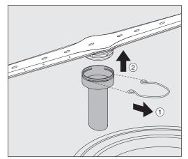
Loosen the securing clip on the spray arm connection and then pull the lower spray arm upwards and the upper spray arm downwards.
