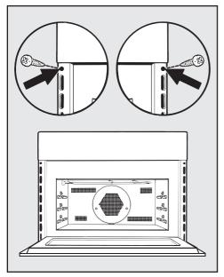
Open the door with the sensor and use the screws supplied to secure the oven to the side walls of the housing unit through the holes in the oven trim.
