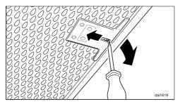
If a grease filter is inadvertently fitted upside down, insert a small screwdriver blade into the slit to disengage the clip.
