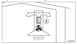
In recirculation mode the silencer needs to be positioned between the exhaust connection and the directional unit ②. Please ensure there is adequate installation space.
