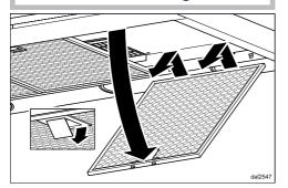
■ To take out the grease filter, release the locking clip on the filter, lower the filter approx. 45°, unhook it at the back and remove it.
