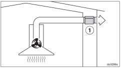
In extraction mode the silencer not only reduces noise from the fan outside the house, but also sounds from outside which reach the kitchen via the vent ducting (e.g. traffic noise). For this reason, the silencer must be positioned as close as possible to the ducting exit ①.
