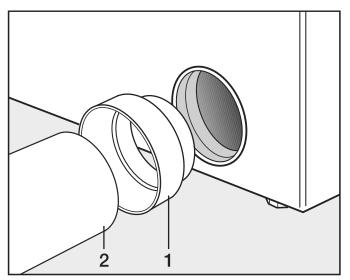
■ Install the connector (1) and the pipe (2).
