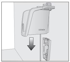
Slide the wall bracket down into the mounting plate from above until it audibly clicks into place.
