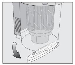
The dust container flap will open and the dust will fall out.
