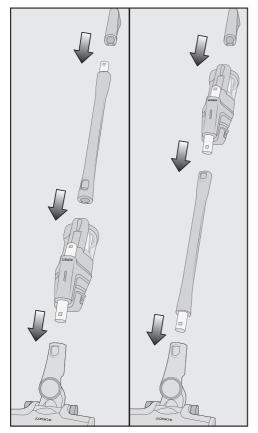
■ You can place the suction tube either above or below the PowerUnit.
