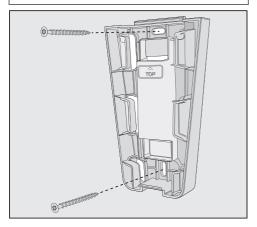
■ Attach the mounting plate to the wall.
