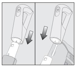
Press the release catch and remove the Comfort handle by pulling it upwards.
