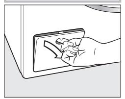
Open the access panel to the drain system.
