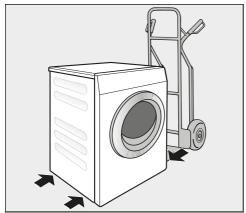
If transporting the washing machine with a sack truck, make sure its left or right side is resting on the truck.
