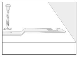
Install the holding bracket with the hexagon screws and the washers.
