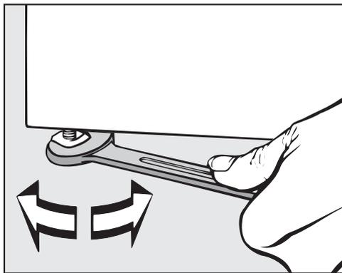
**Tip:** Use a spirit level to ensure correct alignment.
