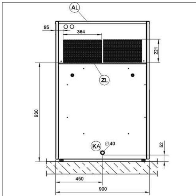
AL Extracted air (air outlet vent)
