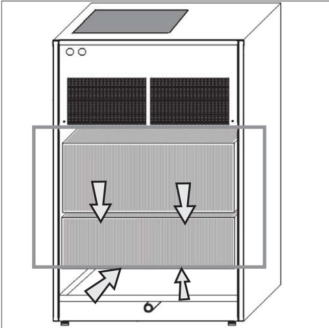
Area of the heat exchangers to be cleaned – behind the service panel (at the back of the machine)
