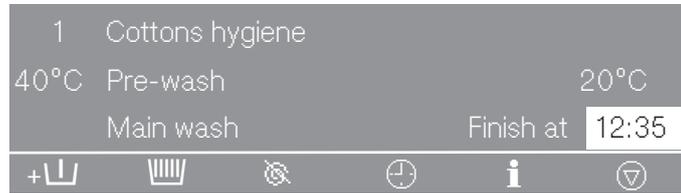
In the second line of the display, in this case Pre-wash, the current suds temperature is shown.
