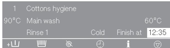
If the Pre-wash programme block is finished, the Main wash programme block will appear in the second line of the display with the current suds temperature. The next programme block, in this case Rinses 1, is shown below.
