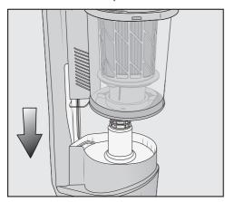
Slide the dust container handle along the guide line and down onto the PowerUnit connector from above until the dust container audibly clicks into place.
