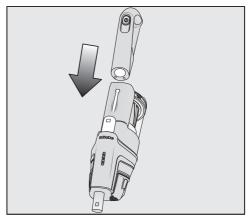
The PowerUnit can be used on its own without the suction tube and electrobrush as a quick way of vacuuming up crumbs and fluff in specific areas.
