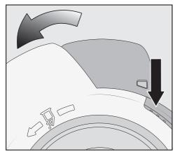
■ Turn the lid of the dust container in the direction of the arrow as far as the first stop. Use the grey gripping surfaces to help you do this.
