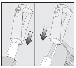
Press the release button and remove the Comfort handle by pulling it upwards.
