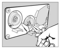
■ Use pointed pliers to grip the bar and pull out the filter; then clean the filter. Reassemble in reverse order.
