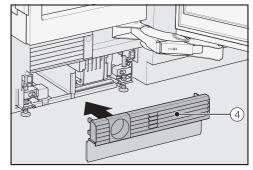
■ Click the plinth ventilation grille ④ onto the bottom of the appliance plinth.
