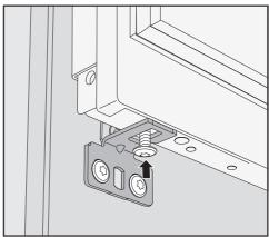
■ Tighten the screw at the bottom of the appliance door.
