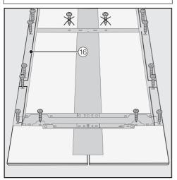
■ For cassette fronts: only secure the mounting frame <sup>(6)</sup> to the outer frame with the screws.
