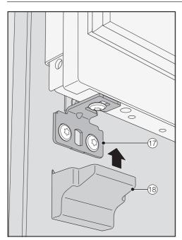
■ Fit the cover <sup>®</sup> over the fixing bracket <sup>1</sup>.
