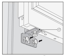
■ Screw the fixing bracket 17 securely to the furniture front.
