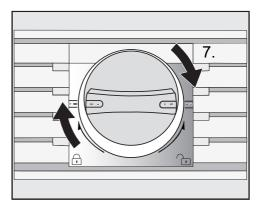
Turn the cap of the filter cartridge clockwise until it is in the horizontal position 7.).
