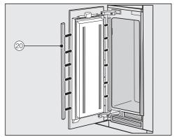
■ Fit the plastic covers ② on both sides of the appliance door by clicking them into the gap between the appliance door and the furniture front, starting at the bottom and working up to the top.
