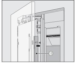
■ Press the angle trims ③ into the white plastic frame on both sides from the outside and screw them on loosely at first. Spare screws are provided in the plastic bag marked with the letter E.
