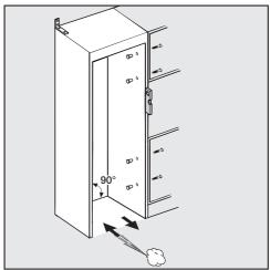
The building-in niche must be carefully aligned using a spirit level before the refrigeration appliance is installed. The niche corners must be at 90° angles to each other, otherwise the furniture front will not sit straight on all 4 corners of the building-in niche.
