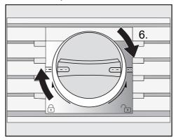
■ Turn the cap of the filter cartridge clockwise until it is in the horizontal position 6.).
