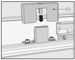
■ Fit the cover ② onto the light contact switch.
