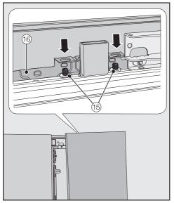
■ Open the appliance door and hang the furniture front on its frame <sup>16</sup> onto the threaded bolts <sup>15</sup>.
