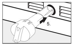
■ Slide the filter cartridge as far as it will go into the filter opening 5.), making sure the cap is vertical.
