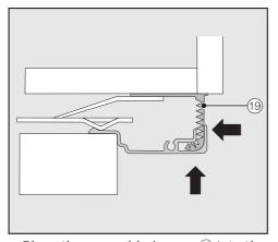
Place the assembled cover (9) into the gap above the refrigeration appliance so it clicks into place. While doing so, slide both parts of the cover together as required.
