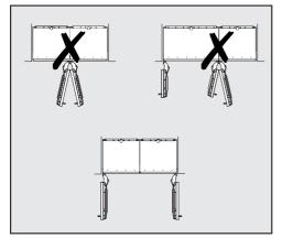
If the refrigeration appliances are to be installed next to each other without a partition wall between them, they will need to be joined together with the side-by-side installation kit. In addition, you must install the side panel heater to prevent condensation from forming and any resulting damage.
