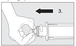
■ Pull the filter out of the back of the filter cartridge 3.).
