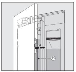
■ Align the depth of the furniture front via the gaps in the angle trims <sup>13</sup>.
