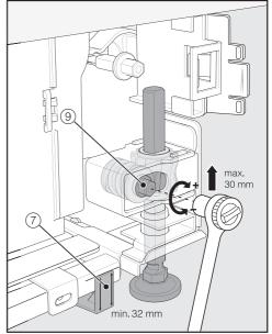
Adjust the front feet with a ratchet (attachment: socket, 8 mm) or a TX 20 screwdriver 9.
