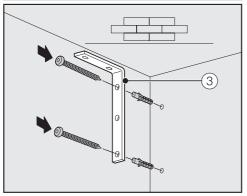
Securing to a concrete wall
