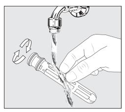
Rinse the filter under running lukewarm water. Turn the filter over under the running water to clean it on all sides.
