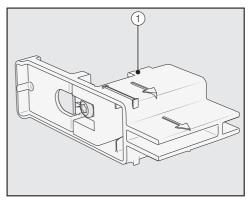
■ Do **not** remove the installation aids ① from the appliance door. These will be required later for aligning the appliance in the building-in niche.
