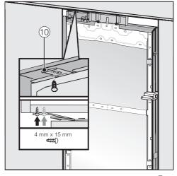
Screw the lugs for the fixing plate <sup>10</sup> into the cabinets/units above the appliance.
