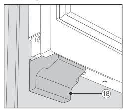
■ Click the cover <sup>®</sup> onto the fixing bracket.
