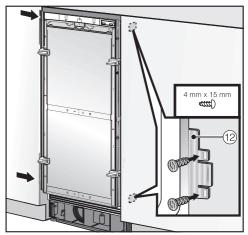
■ Screw the fixing plate lugs <sup>12</sup> at the top and bottom to the cabinets/units adjacent to the appliance.
