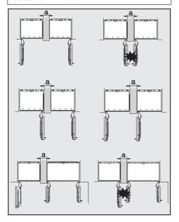
If the door hinges of the refrigeration appliances are next to each other, you must take into account the thickness of the furniture fronts and door handles so that the appliance doors do not collide and become damaged if they are opened at the same time.
