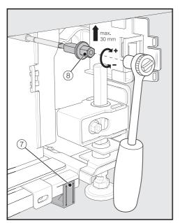
Adjust the rear feet with a ratchet (attachment: socket, 8 mm) or a TX 20 screwdriver <sup>(8)</sup>.
