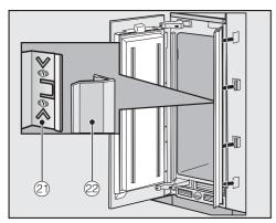
Now attach the covers ② onto the retaining clips ③ on each side. In the case of side-by-side installation, the covers are only required on the outer side.
