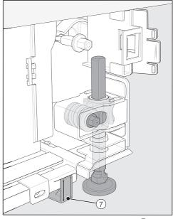
■ Position the supplied spacers ⑦ on both sides on the markings next to the adjustable feet at the front of the refrigeration appliance.
