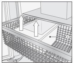
Tilt the ice cube container 4 forwards and pull it up and out to remove it. Ice cube production does not stop when the ice cube container has been removed. Ice cubes can fall into the freezer basket underneath.
