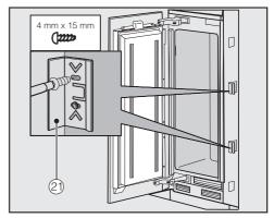
Secure both sides of the refrigeration appliance using at least 3 clips (2) for the covers.
