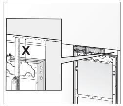
■ Measure the gap **X** between the mounting frame and the upper edge of the adjacent furniture front.
