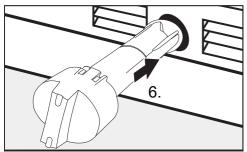
Slide the new filter cartridge as far as it will go into the filter opening 6.), making sure the cap is vertical.
