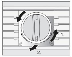
■ Turn the cap of the filter cartridge anti-clockwise until it is in the vertical position 1.) and slide it out of the filter opening 2.).
