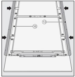
■ Now insert the angle trims ③ on both sides as far as they will go into the provided spaces in the mounting frame ⑥.
