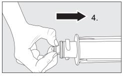
■ Reinsert the filter into the back of the filter cartridge 4.).
