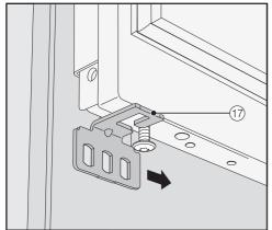
■ Slide the fixing bracket ⑦ sideways onto the screw at the bottom of the appliance door.
