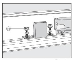
■ Place the washers and nuts ⑭ back in position and tighten the nuts ⑭. The furniture front is now secured.
