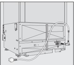
■ Insert the plug connector into the socket at the back of the refrigeration appliance.
