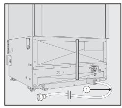
The stainless steel hose for the refrigeration appliance ① is ready for connection at the rear of the appliance.
