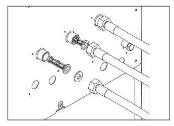
■ Check and clean regularly the filters in the water intake faucets, and the water intake hoses.
