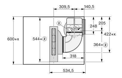
If you want to install the air duct to the left of the downdraft extractor, the work-top must be at least 665 mm deep.
