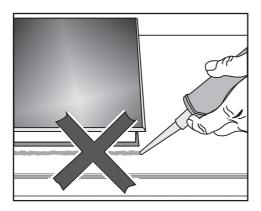
The SmartLine element and worktop may be damaged if the element needs to be removed after it has been sealed with a sealant. Do not use any sealant between the SmartLine element and the worktop. The seal under the edge of the top part of the appliance provides a sufficient seal for the worktop.
