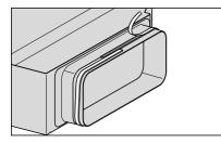
If the exhaust ducting does not sit securely up against the exhaust duct connection, stick the sealing strip supplied to the exhaust duct connection.
