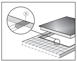
Grout lines ① and the hatched area underneath the SmartLine element frame must be smooth and even. If they are not, the SmartLine element will not sit flush with the worktop and the sealing strip underneath the top part of the appliance will not provide a good seal between the appliance and the worktop.
