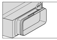
If the exhaust ducting does not sit securely up against the exhaust duct connection, stick the sealing strip supplied to the exhaust duct connection.
