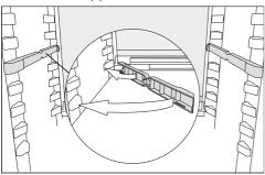
Attach the two adapters to the support ribs on the left and right at the desired height.
