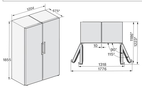
\* Dimensions without wall spacers fitted. Appliance depth is increased by 15 mm with the wall spacers supplied fitted.
