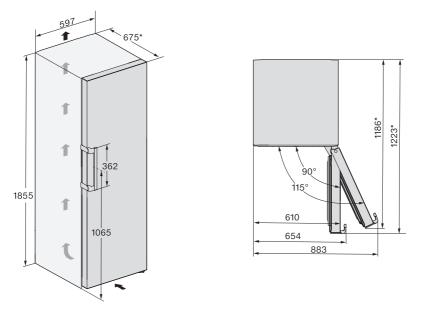
$^{\ast}$  Dimensions without wall spacers fitted. Appliance depth is increased by 15 mm with the wall spacers supplied fitted.
