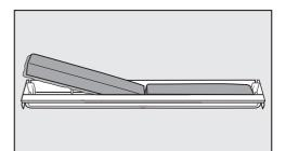
Remove both charcoal filters and place the new filters with the surrounding edge pointing downwards in the holder.
