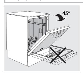
■ Open the door to an angle of around 45°. This ensures that the salt flows into the salt reservoir more easily.
