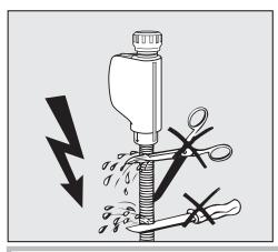
1 Do **not** shorten or otherwise damage the inlet hoses supplied with the machine.
