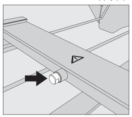
Under no circumstances may items to be washed, washing attachments etc., be connected to the test point. After the measurement, the test point must be closed again with the blind stopper.
