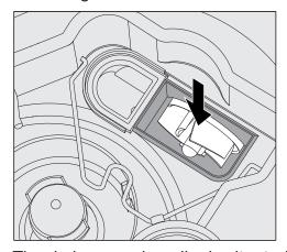
The drain pump impeller is situated under the non-return valve (see arrow).
