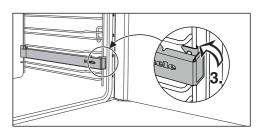
■ Then secure the telescopic runner to the bottom of the two rails as illustrated (3).
