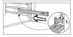
■ Hook the FlexiClip telescopic runner onto the bottom rail of a shelf level at the front (1.) and push it along the rail into the oven interior (2.).
