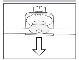
Carefully pull down the pressure cap. The top heat/grill element then lowers automatically.
