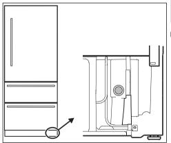
Gently push the appliance into the desired location. Leave enough space behind the appliance for connecting the water supply.
