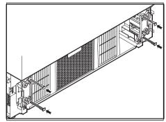
Insert the locking pins on both sides to secure the retainers in the appliance housing.
