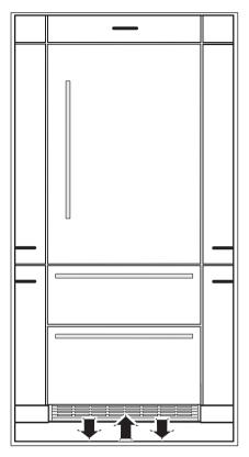
This appliance does not require ventilation openings in the surrounding cabinetry. Proper ventilation is ensured though the ventilation slits at the base of the appliance.
