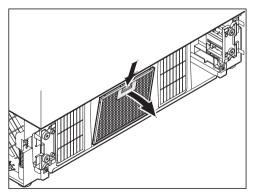
Push the latch of the air filter downwards and take it out.
