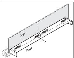
Securing with angular positioning of the screws (1/4" x 2 1/2") (6 x 63 mm) С
