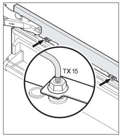
To vertically align the door panel with the adjacent cabinet doors,
