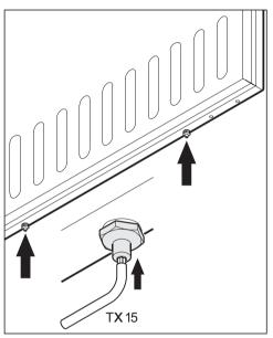
Screw the adjustment bolts on the lower side of the appliance door as far as possible into the door.
