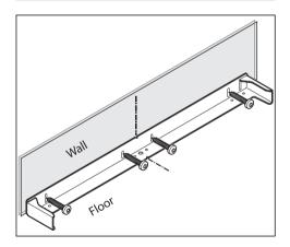
Mark the center line of the appliance on the back wall of the installation niche. The center of the anti-tip bracket must be aligned with this line.
