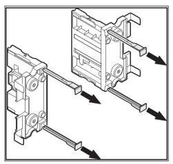
Remove the locking pins from the supplied retainers.
