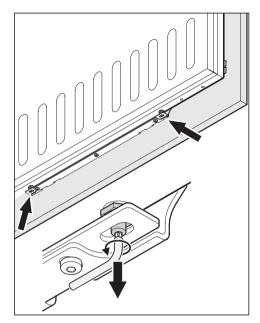
Tighten the adjustment bolts on the lower side of the appliance door until the mounting rail sits tight on the appliance door.
