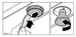
Insert the lever supplied into the gap between the lamp and the lamp holder.
