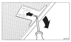
If a grease filter is inadvertently refitted upside down, insert a small screwdriver blade into the slit to disengage the clip.
